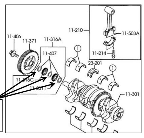
Crankshaft Friction Disc, 3 Required For Turbo Engines. Crankshaft Friction Disc, 2 Required For Non Turbo Engines.
