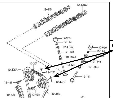
Variable Valve Timing Friction Disc two pieces required.
