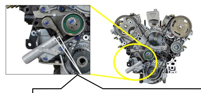
Due To The OE Manufactures Procedures Required In The Installation Of New Timing Components, NASON Strongly Recommends That All Installers Check The Hydraulic Tensioner Rod Protrusion After Completion.
