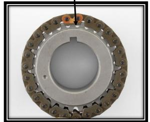
NTC1200: Note the installed chain position, as per the OEM chain
