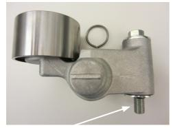
Apply Threadlocker to tensioner pivot bolt threads prior to installation.
