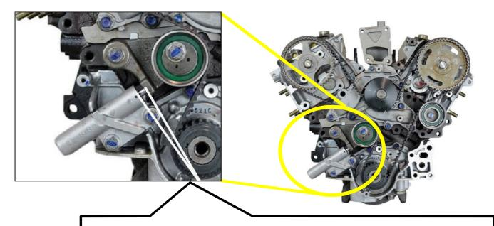
Due To The OE Manufactures Procedures Required In The Installation Of New Timing Components, NASON Strongly Recommends That All Installers Check The Hydraulic Tensioner Rod Protrusion After Completion.
