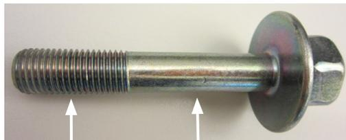
**Inspect the crankshaft pulley bolt and threads for ANY Indication of Stretching!**
