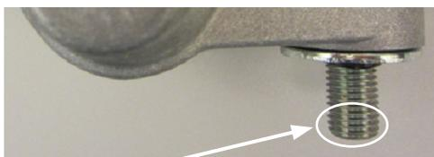
**Apply several drops of Threadlocker to the first few threads.**
